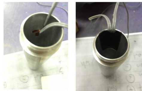
Fig.2 Strain gauges by full Wheatstone bridge circuit
